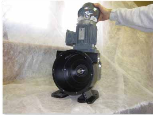
Figure 4: Remove Motor Fan Cover
