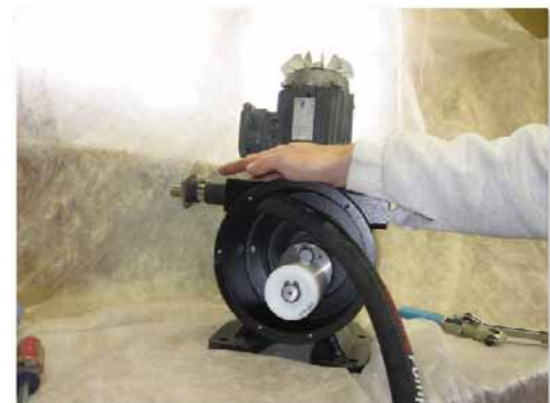
Figure 13: Bandit Clamp Installed
