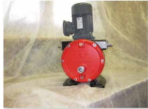
Figure 29: A Newly Rebuilt Eccentric Pump
