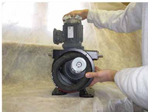
Figure 20: Turn Roller to the Twelve O'clock
