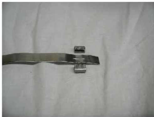
Figure 30: Band-it Clamp Cut with a Hack Saw
