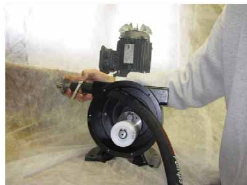
Figure 12: Assembly of Bandit Clamp and Barb
