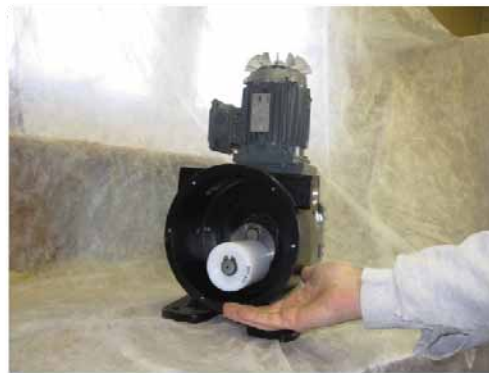
Figure 31: Hose Freed from Roller and Pump
