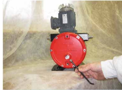
Figure 25: Installing the Drain Plug
