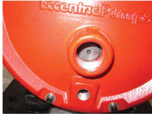
Figure 24: Roller Viewed through Sight Glass at Six O'clock Position
