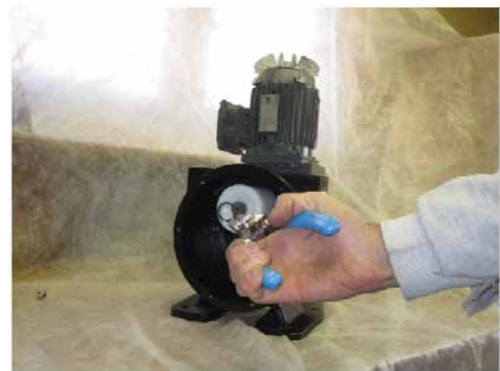
Figure 9: Installation of Roller Retaining Clip
