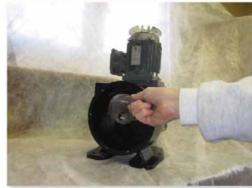
Figure 35: Removal of the Eccentric Shaft
