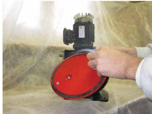
Figure 22: Aligning the Gasket on the Front Cover
