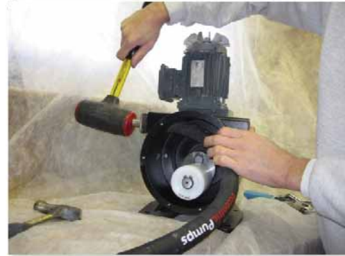
Figure 15: Using a Dead Blow Hammer to Help Seat the Barb Assembly
