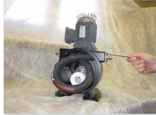
Figure 19: Installation of Second Barb Assembly Bolts
