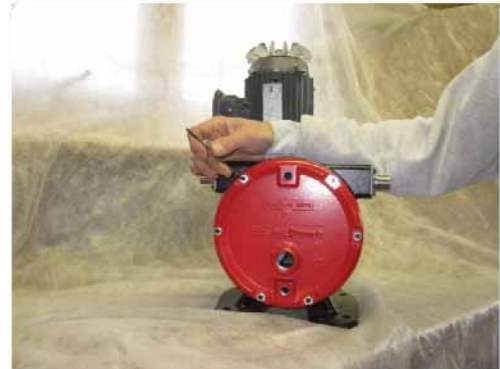
Figure 23: Tightening the Front Cover
