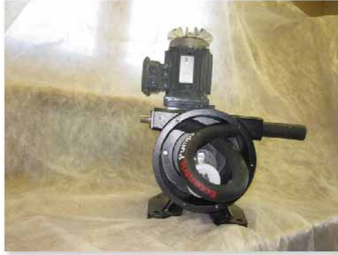
Figure 18: Installation of Hose Through Front Opening
