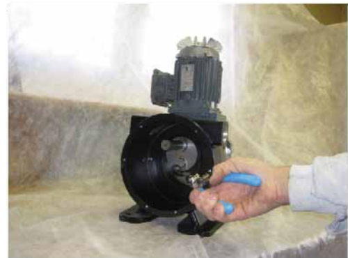
Figure 7: Installation of Eccentric Shaft Retaining Clip
