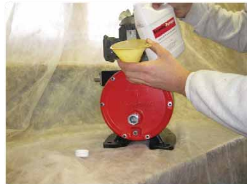
Figure 27: Filling the Pump with Hoselube
