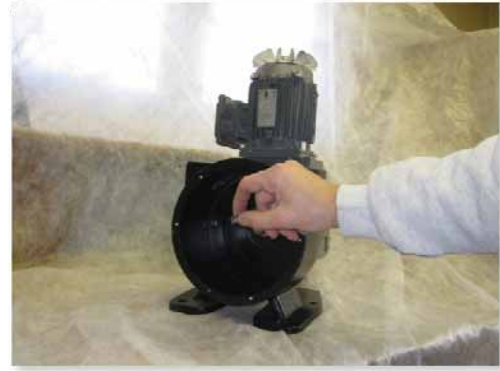
Figure 5: Installation of Eccentric Shaft Key
