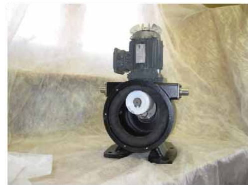
Figure 21: Seating of the Hose with the Roller in the Twelve O'clock Position
