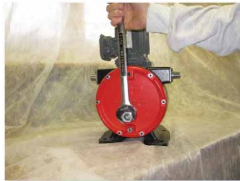
Figure 26: Installation of Sight Glass
