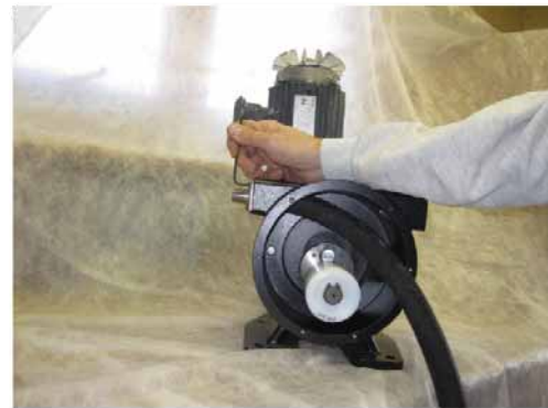
Figure 17: Tightening Socket Head Cap Screws
