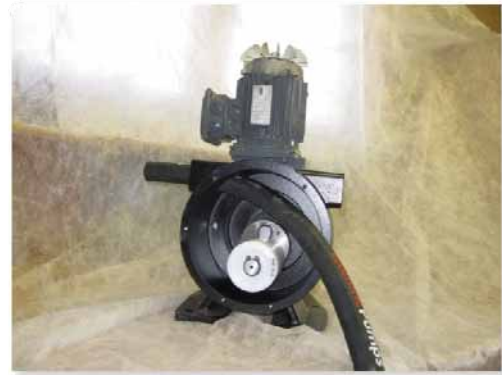
Figure 11: Pass Hose Through the Rear Opening of the Pump Body
