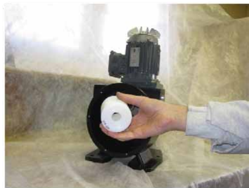
Figure 8: Installation of Roller on to Shaft
