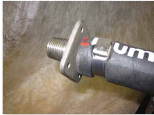
Figure 14: Bandit Clamp Approximately 3/8" (9.5mm) from Back of Barb
