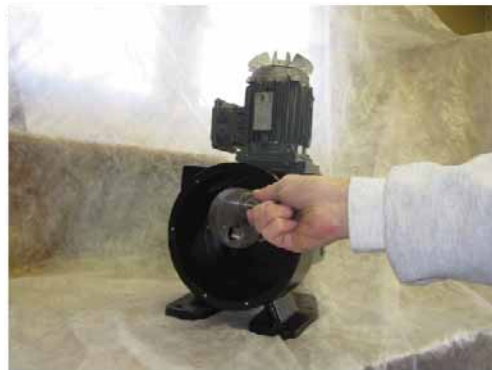
Figure 6: Place the Eccentric Shaft on the Main Pump Shaft
