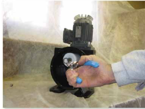
Figure 32: Removal of Roller Retaining Clip
