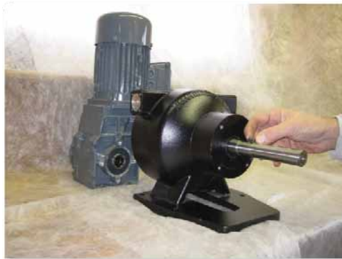
Figure 2: Insert Key(s) in the Shaft
