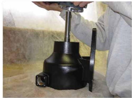
Figure 3: Installation of Gearbox
