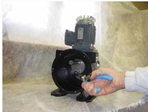
Figure 34: Removal of Eccentric Shaft Retaining Clip
