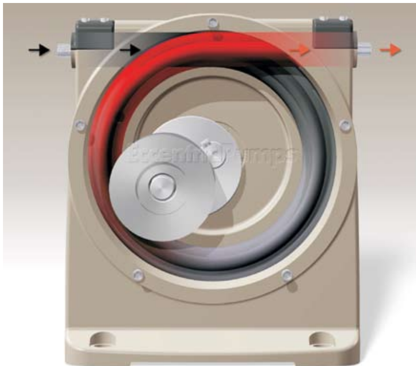
Figure 1. The positive displacement pump used in the trials. The full 360 degrees of hose allow more flow per revolution and fewer pulses than hoses arranged in a C-shape.
